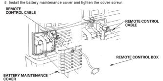
9. To avoid accidentally unplugging the remote control cable, secure the cable to the generator frame with a cable tie as shown.
