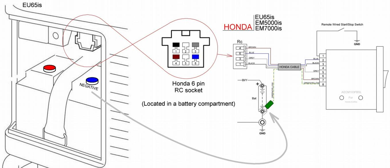
To fit the module using our Honda eu65is cable:
