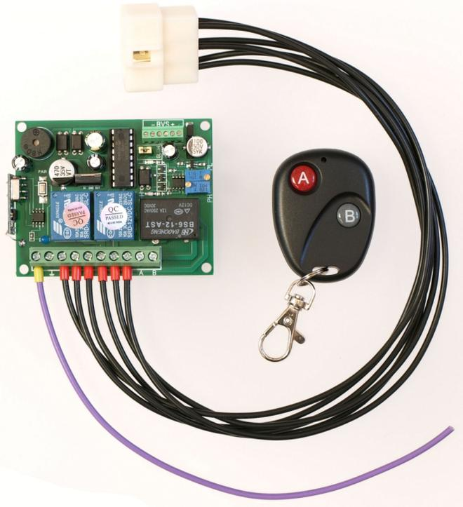
To reset the ATS controller after the engine failure was identified and fixed: press button "B" on your key fob or, if the engine was initially started from the ATS panel connected to the 3 pin ATS socket – disconnect the 3 pin plug and/or switch off the "generator start" request from ATS panel connected to it. If the engine run was initially triggered by the BVS (battery voltage sensor) – please disconnect at least 1 wire connected to the BVS terminal.
