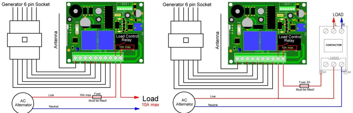
For the load current 10A or less it is possible to use the Load Control Relay fitted on the ATS controller. If the load is greater than 10A please use an appropriately rated contactor.
