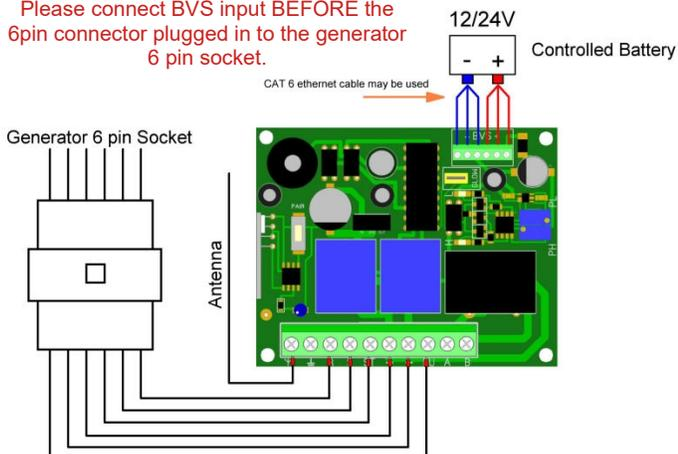
Battery Voltage Sensor — this internally fitted device intended to automatically control your battery voltage. Should the controlled battery voltage drops below the set threshold, the BVS will then initiate a start command sending a signal to the ATS controller. The generator will run until the BVS senses the battery high voltage threshold. The low and high voltage thresholds are:
